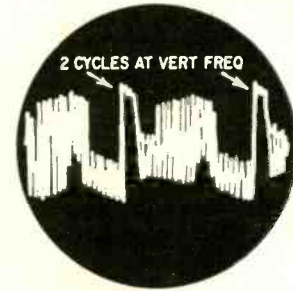
Fig. 3—Two cycles of video at 30-cycle sweep. Look for the vertical sync pulses.
