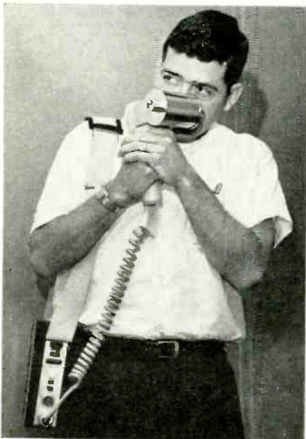
Fig. 10—Short-range laser can be hand-held.
