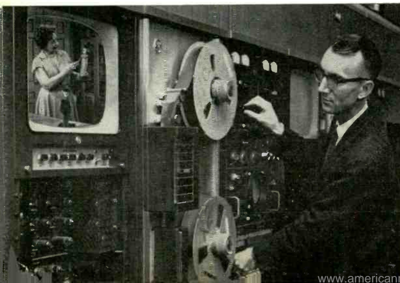
At class time, tape is played back and fed into closed-circuit system. Technicians monitor the program at all times.
