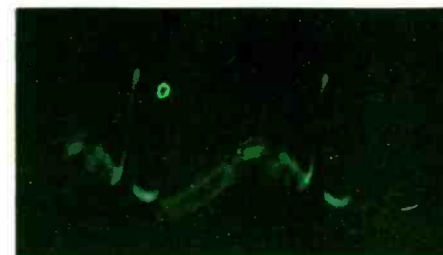
Fig. 8—Outline of 60-cycle hum voltage is evident in this pattern.
