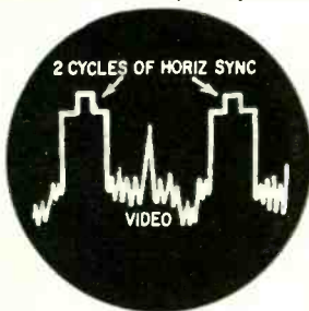
Fig. 1—Two cycles of horizontal sync on the scope screen.
