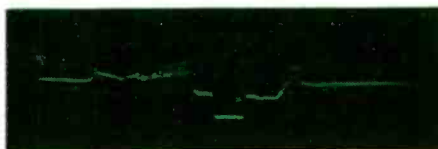
Fig. 3—Horizontal sync pulse at output of video amplifier in receiver.
